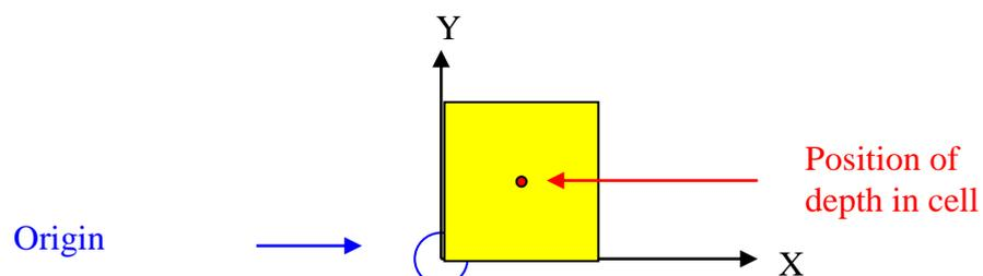
In order to avoid interpolation of the 30 arc-second GEBCO grid values, rows and lines of the EMODnet DTMs must be aligned with rows and lines of the GEBCO grid as illustrated below :
