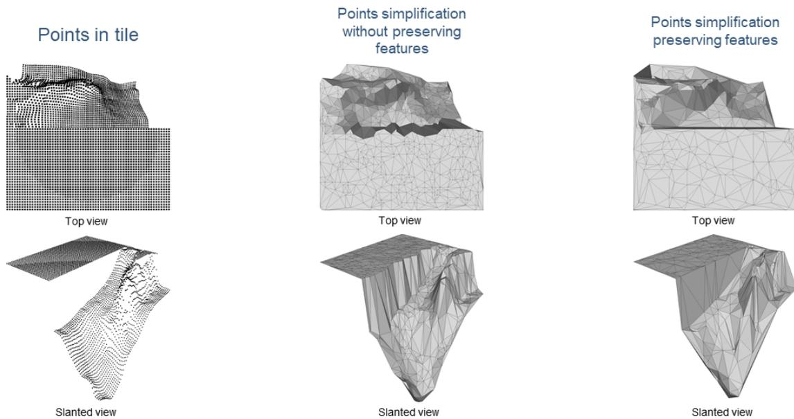
*Figure 4. Point set simplification. We find the original point set on the right. In the middle, one can see the result of applying a point set simplification to the points directly. You can observe how the square shape of the tile is corrupted, and how the vertical “cliff” is not preserved. By using our two-steps method, as visible in the right part of the figure, we preserve the straight boundaries of the tile, as well as the sharp features present in the original data.*
