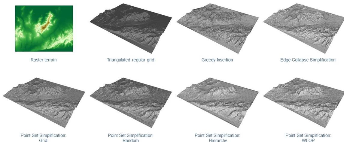
*Figure 5. From left to right, top to bottom, we can see the original raster as an image, the result of triangulating all the samples in the terrain (and the huge number of triangles that this produces), and then the result of applying the different simplification methods studied in*
