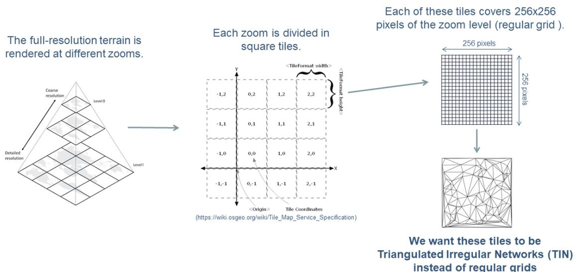
*Figure 1. Overview of the proposed methodology. We aim at creating a multi-resolution tiled representation of a terrain as the one shown on the left hand side. Each of the LOD (also called zooms) is tiled following a regular grid. As shown on the right hand side, each of these tiles covers a 256x256 footprint of a raster file, and we aim at converting this regular*
