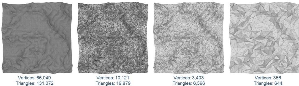
*Figure 2. Different levels of detail of a tile using the edge collapse method. Notice how the reduction in complexity adapts the geometry to the variance in the input terrain, and how in all the cases our modifications preserve the square shape of the tile.*
